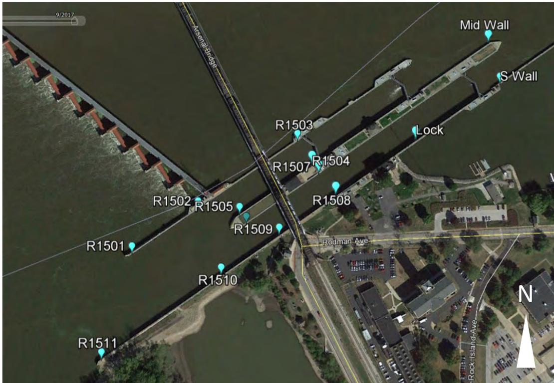
Figure 3. Location of receivers (blue dots) completing the VEMCO receiver array in the lock and lock approaches at Lock and Dam 15. Array maintained by U.S. Geological Survey and Illinois Natural History Survey.
