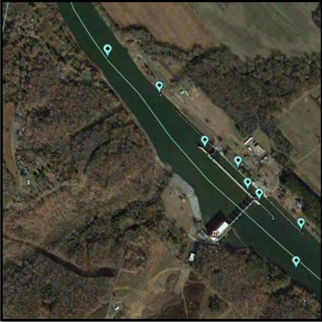
Figure 6. VEMCO telemetry array deployed at Cheatham Lock and Dam.
