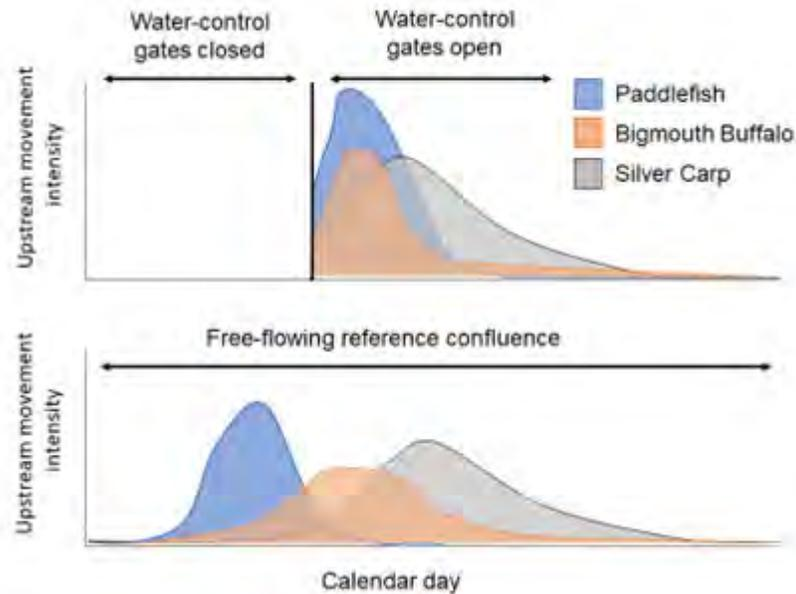
Figure 1: Predicted influence of a water-control structure on upstream movements of Silver Carp, Paddlefish, and Bigmouth Buffalo. When closed, water-control structures synchronize the timing of large-scale movements by allowing passage only when the water-control structure is opened. In an unobstructed confluence, seasonal upstream movements for spawning by native planktivores and Silver Carp coincide lightly.
