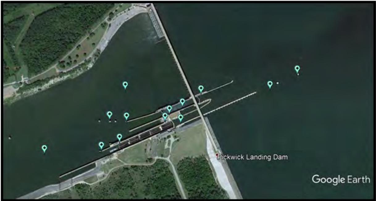
Figure 5. VEMCO telemetry array deployed at Pickwick Lock and Dam.
