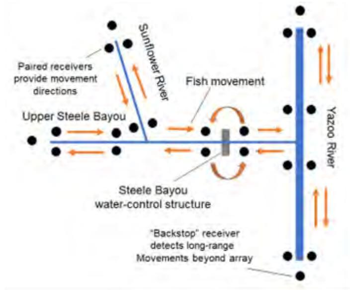
Figure 3. Existing acoustic array spanning Steele Bayou water-control structure in the lower Yazoo River basin. The array monitors movements upstream Yazoo River into Steele Bayou/Sunflower River and through the water-control structure. Backstop receivers will be placed upstream and downstream of the array to monitor long-range movements throughout the Yazoo River system.
