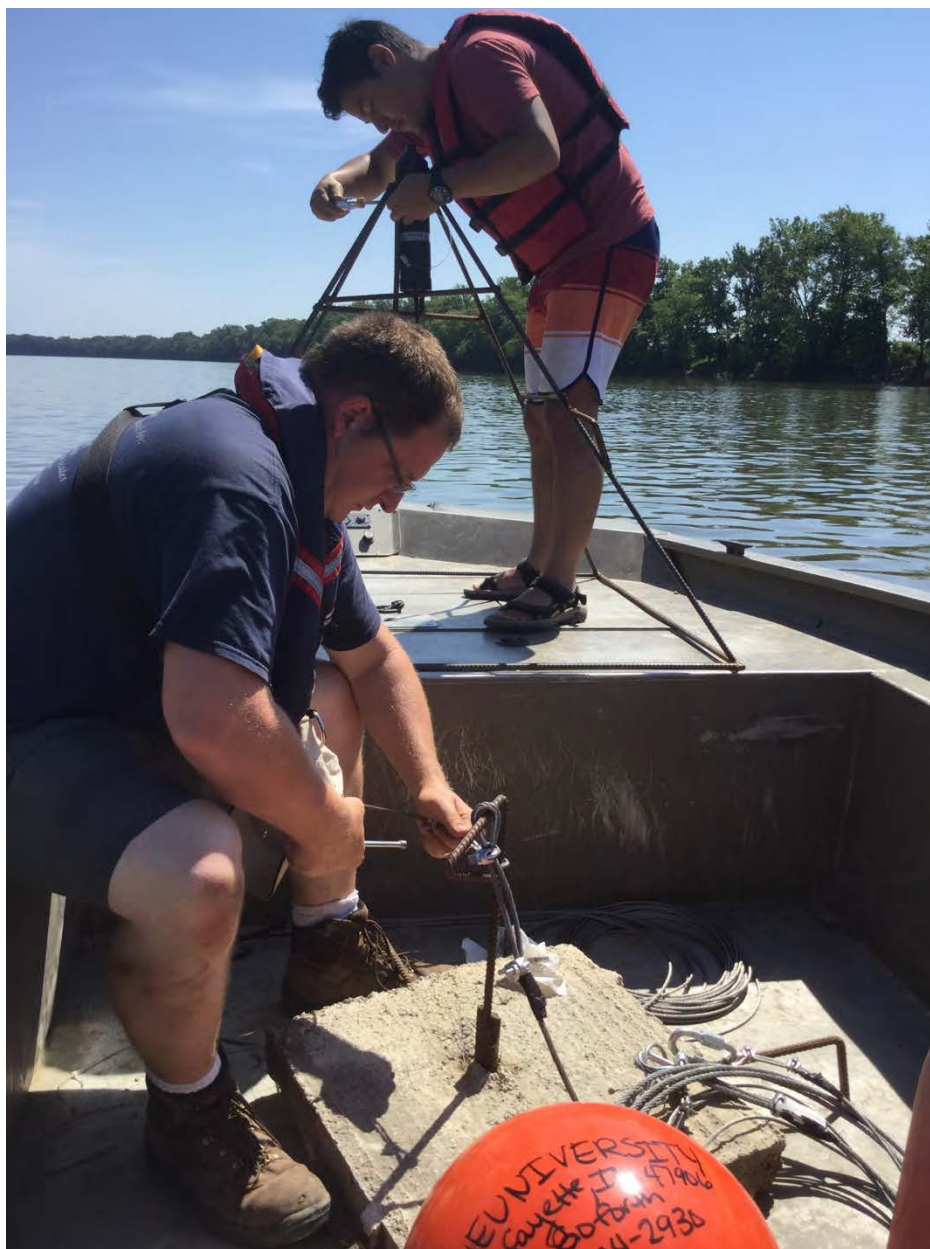
Plate 2. Rebar platform and reinforced concrete anchor system for deploying Vemco VR2W stationary receivers in the lower Wabash River, Indiana.
