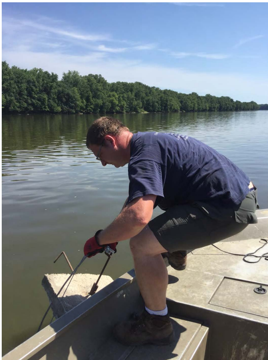
Plate 3. Placing the upstream anchor as part of the platform-anchor system for deploying Vemco VR2W stationary receivers in the lower Wabash River, Indiana.
