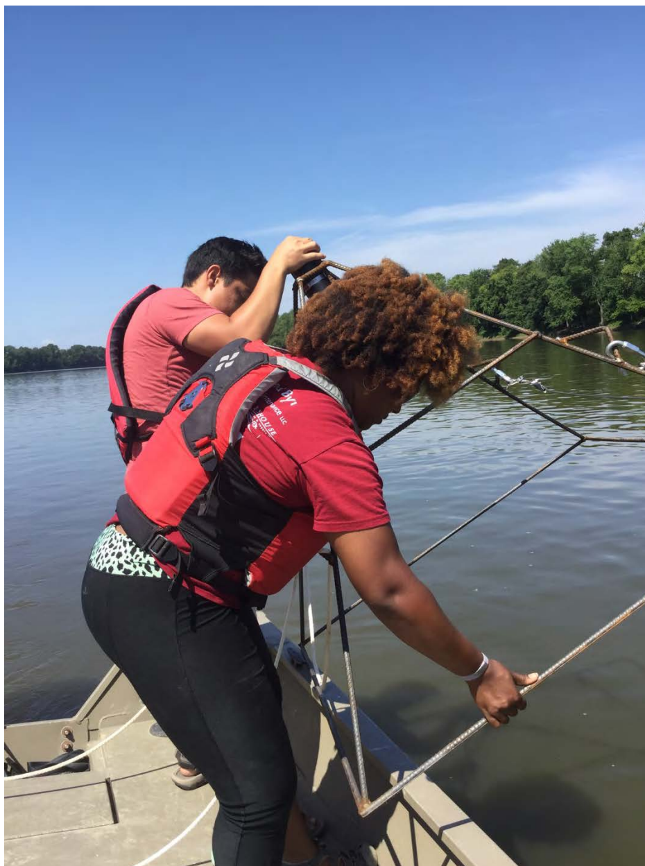
Plate 4. Placing the downstream platform as part of the platform-anchor system for deploying Vemco VR2W stationary receivers in the lower Wabash River, Indiana.
