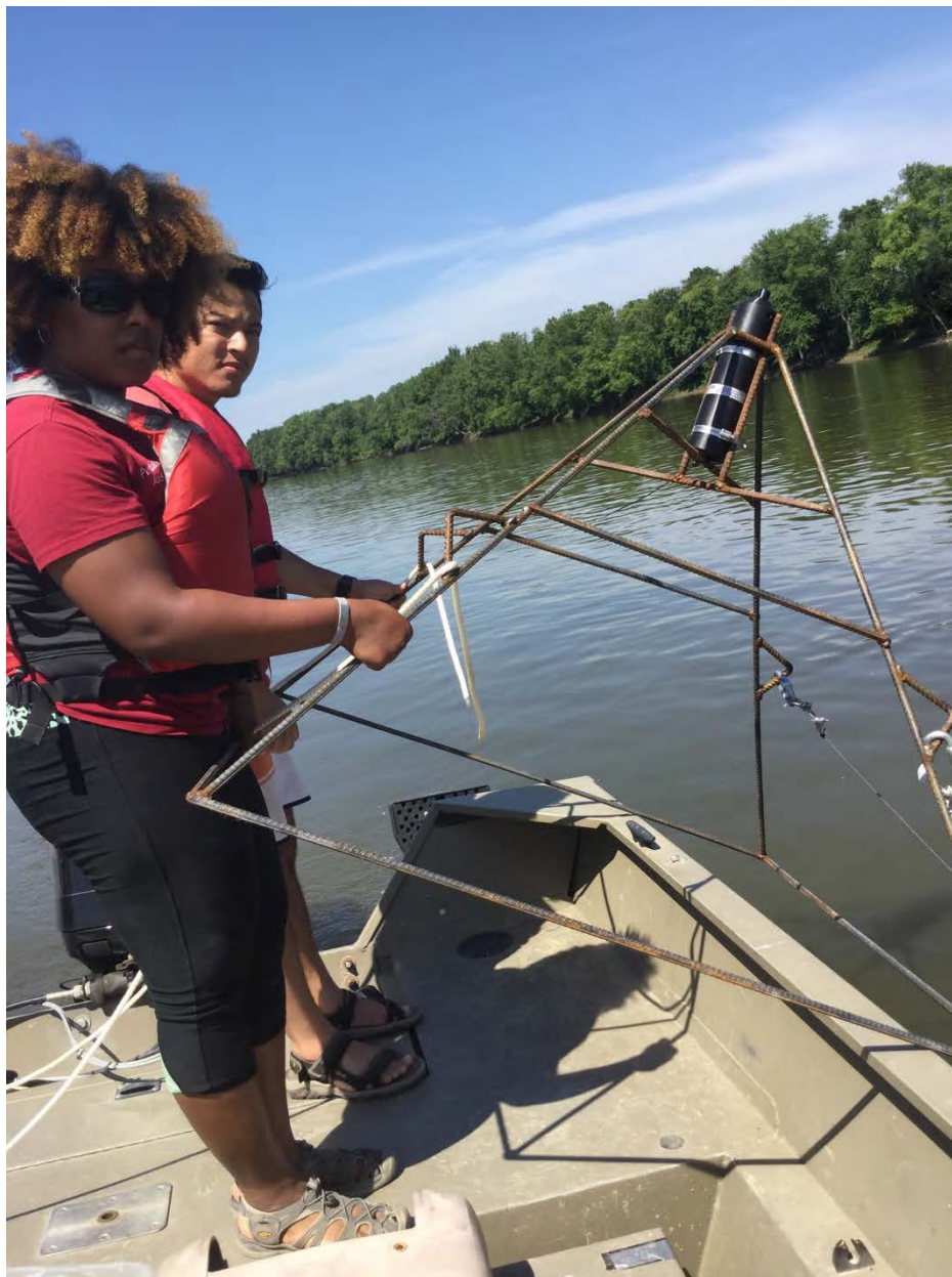
Plate 1. Platforms constructed from 3/8” rebar for deploying Vemco VR2W stationary receivers in the lower Wabash River, Indiana.
