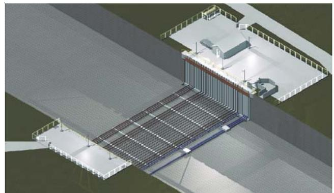
**Diagram of the aquatic nuisance species (ANS) barrier located in the connecting canals between Lake Michigan and the Illinois River. Electric cables laid along the channel bed create an underwater electrical field designed to repel fish.**
