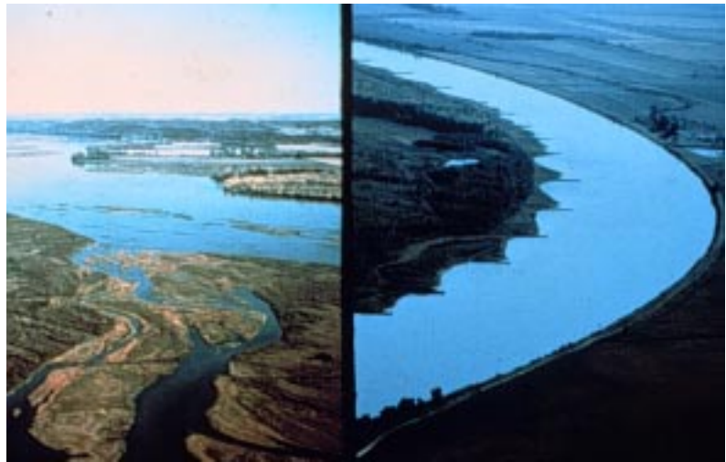
Figure 27. A comparison between a natural river (left) and a channelized river or a “river on drugs” (right).
